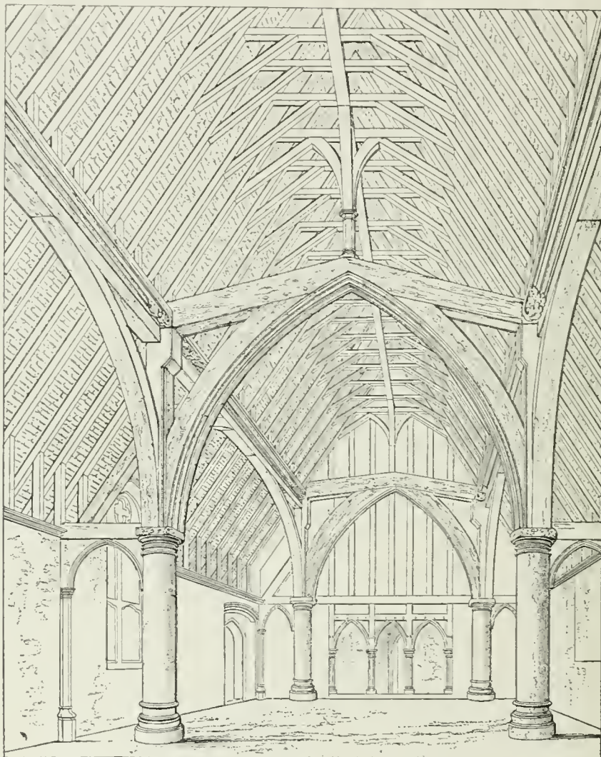
WOOD, CONSTRUCTION IN, PART I., FIG. 1: INTERIOR HALL OF NURSTED COURT, KENT; 13TH CENTURY.
